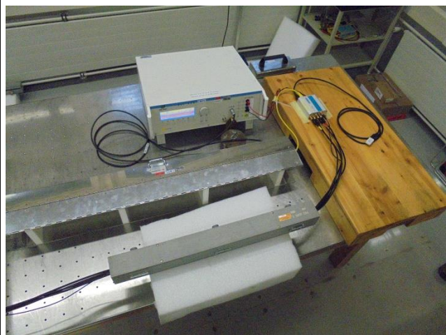
Coupling with clamp (Ethernet)
