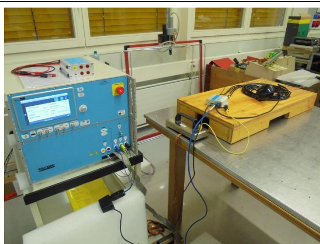
Coupling on AC power port of power adapter
