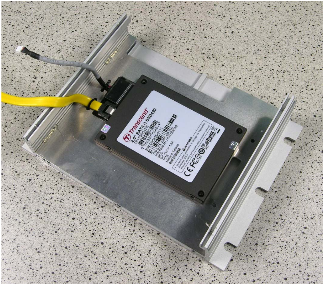
Mainboard removed, solid state drive mounted on bottom plate
