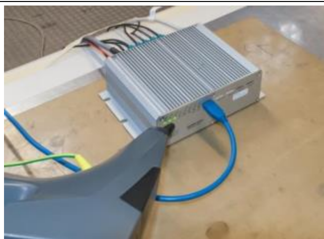
Air Discharge on LED's
