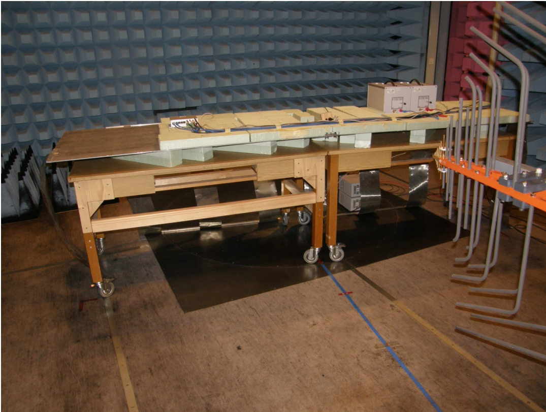
Photo 9: Measurement set-up for radiated Immunity, Log-periodic-antenna
