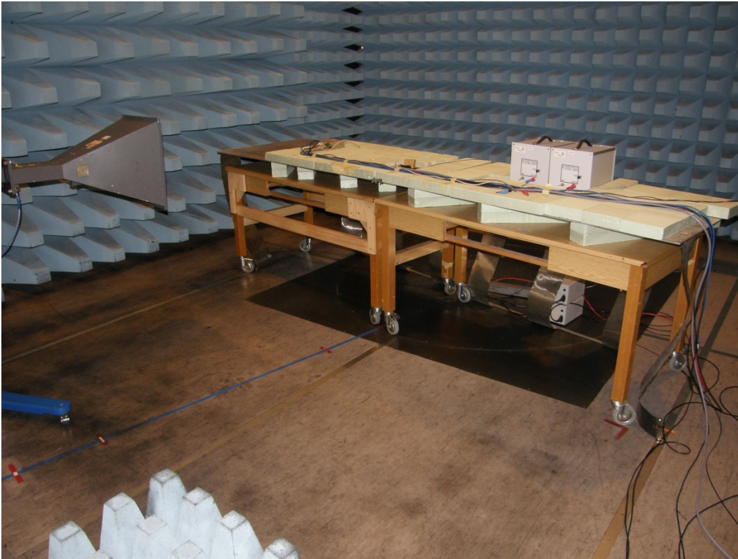
Photo 11: Measurement set-up for radiated Immunity, Horn antenna, for immunity above 1 GHz
